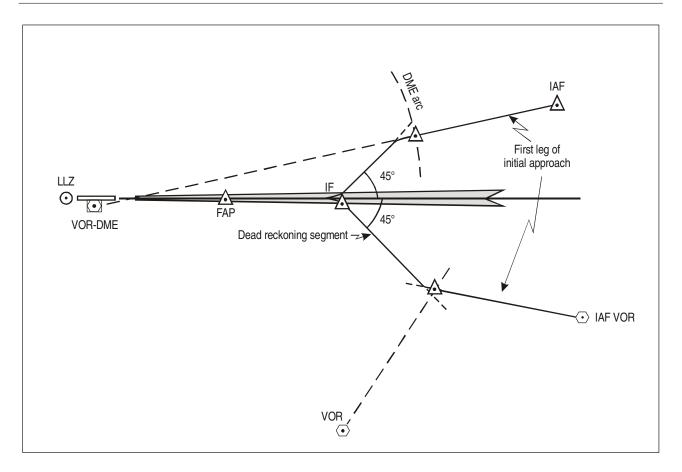
Figure I-4-3-App A-2. S-type procedure
