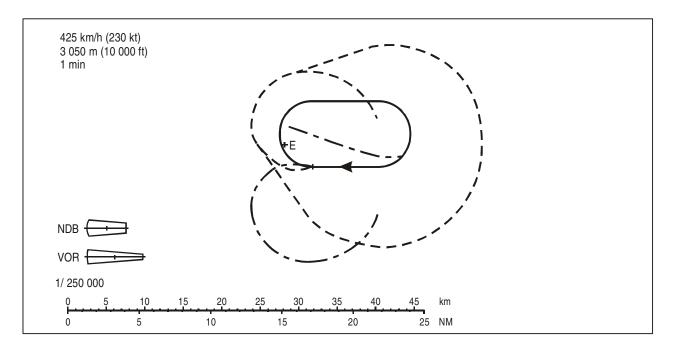
Diagram I-4-3-App C-7. Holding template extracted from the *Template Manual for* Holding, Reversal and Racetrack Procedures (Doc 9371)
