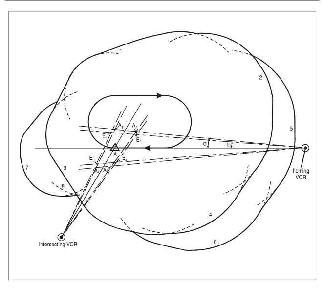
Diagram I-4-3-App C-14. Procedure at the intersection of VOR radials — Basic area and the associated entry area assuming entries along the procedure track and intersecting radial
