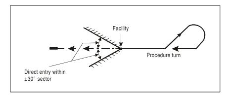
Figure I-4-3-4. Entry to procedure turn
