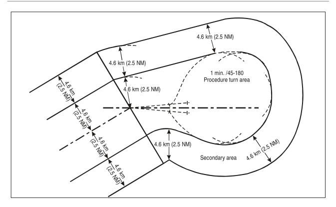
Figure I-4-3-App C-6. Interface between initial segment areas and procedure turn areas
