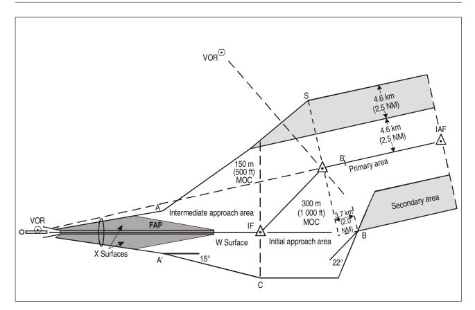
Figure I-4-3-App A-5. S-type VOR/VOR procedure construction of protection areas
