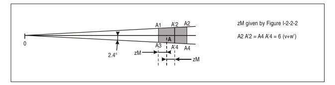
Figure I-4-3-App C-5. Localizer at 0 and marker at A
