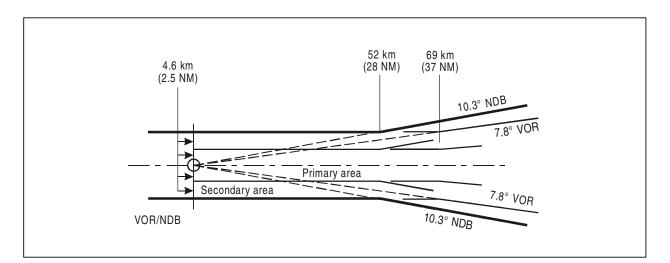
Figure I-4-3-3. Initial approach area utilizing straight tracks
