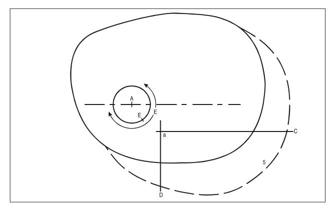
Diagram I-4-3-App C-10. Construction of the entry area; use of point E, the axis of the template being parallel to the procedure axis
