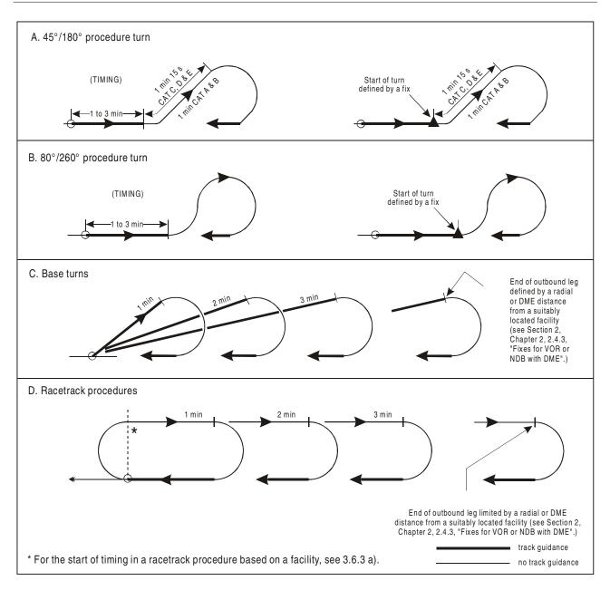
Figure I-4-3-7. Types of reversal and racetrack procedures
