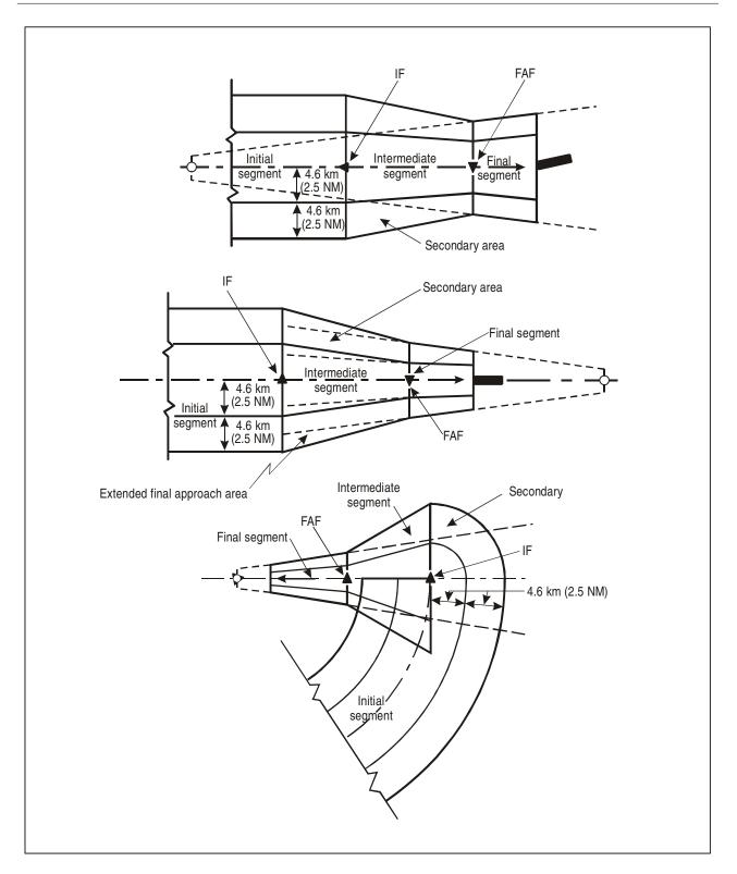
Figure I-4-3-2. Typical segments (plan view)
