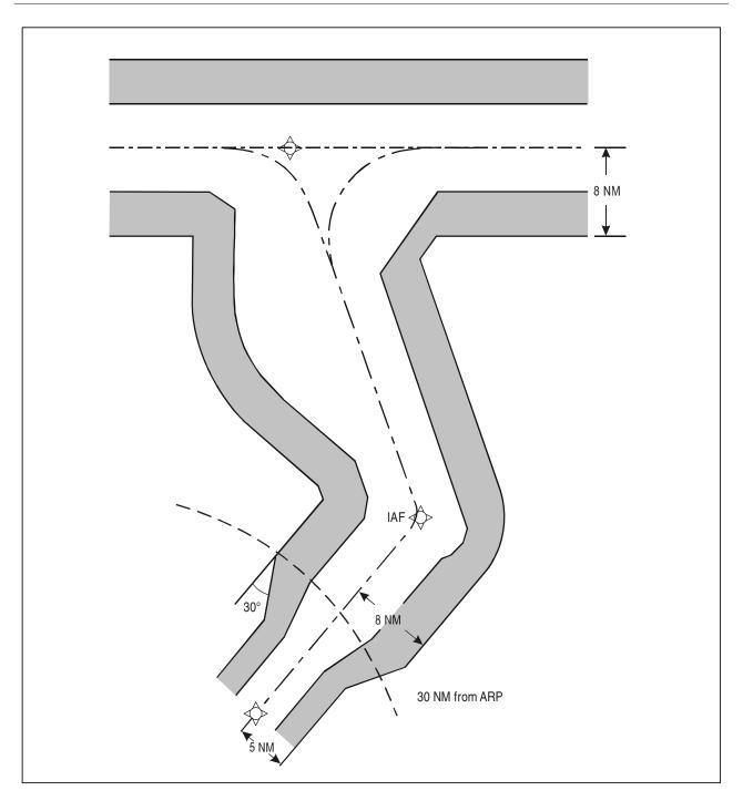
Figure I-4-2-5. GNSS arrival criteria, IAF beyond 30 NM ARP: 8 NM ½ AW prior to 30 NM from ARP then 5 NM ½ AW
