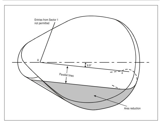
Diagram I-4-3-App C-13. Area reduction for a procedure overhead an NDB when entries from Sector 1 are not permitted
