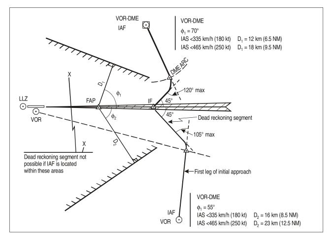
Figure I-4-3-App A-1. U-type procedure conditions for locating the IAF
