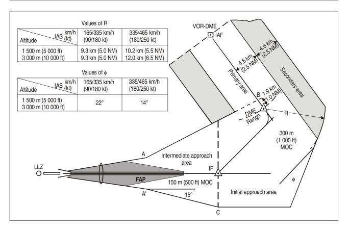
Figure I-4-3-App A-4. U-type VOR/DME procedure construction of protection areas
