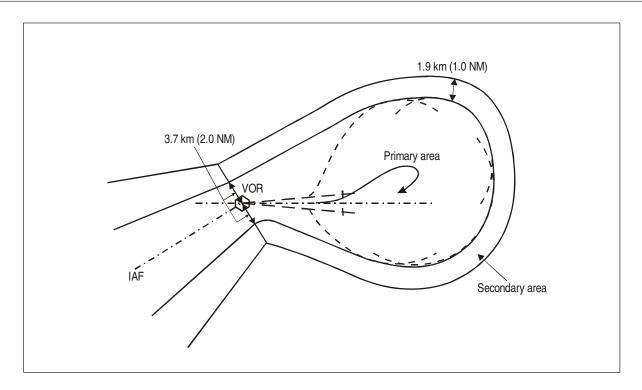
Figure I-4-3-App B-9 Interface between primary and secondary areas of initial approach and reversal procedures (example with a VOR)
