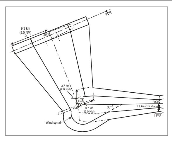
Figure I-4-3-App B-8. Reduction in area widths — initial segment jointed to intermediate segment by a turn
