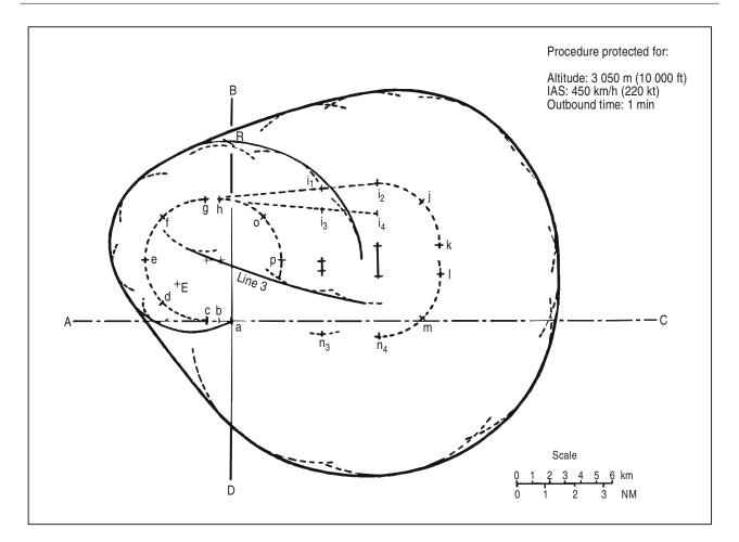
Diagram I-4-3-App C-6. Holding/racetrack template with associated construction points
