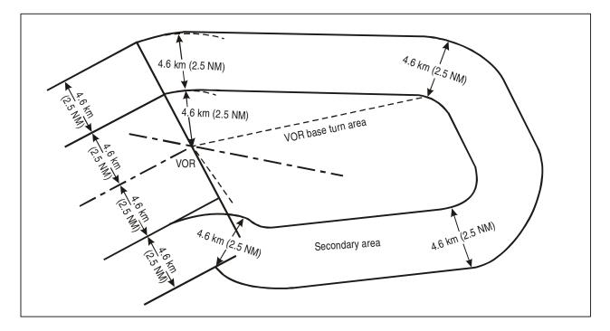
Figure I-4-3-App C-7. Interface between initial segment areas and base turn areas
