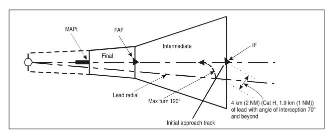
Figure I-4-3-1. Lead radial for turns greater than  $70^{\circ}$
