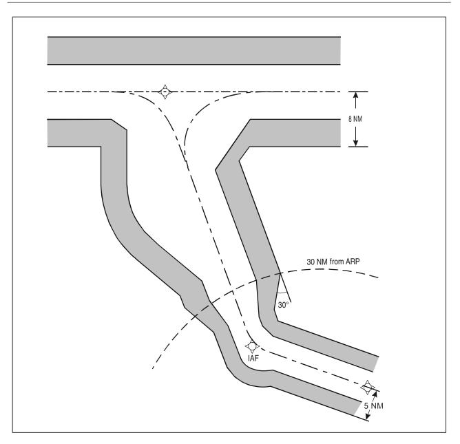
Figure I-4-2-6. GNSS arrival criteria, IAF within 30 NM ARP: 8 NM ½ AW prior to 30 NM (46 km) from ARP then 5 NM ½ AW
