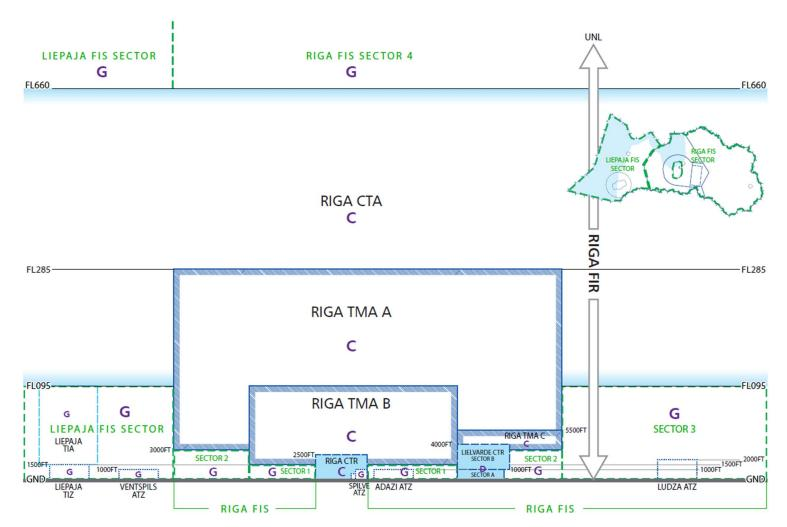
4.2 Fig. Airspace structure of the Republic of Latvia in the vertical plane<sup>7</sup>
