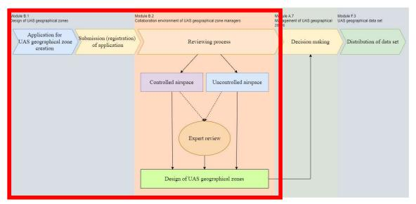
6.3 Fig. Stages of the UAS geographical zone establishment process in Block B
